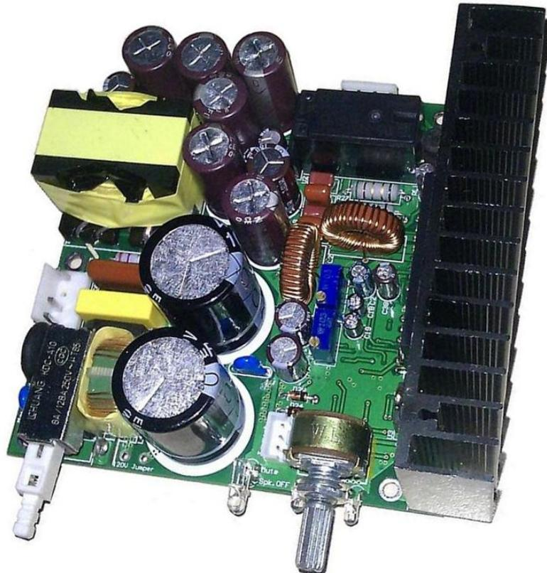
**Figure 1: TA2022SMPS Audio Amplifier Module**
